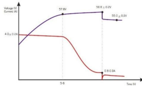
**Phase 1:** The Max. charge current is 4A, and the charge voltage is gradually risen up to 57.6V;
